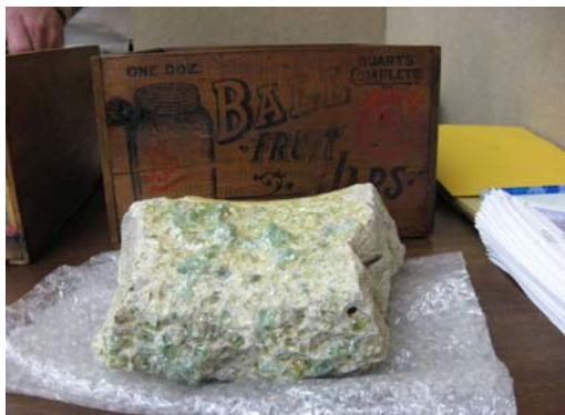
Lou Ebert brought this chunk of a glass melting pot from the site of the Marion Fruit Jar & Bottle Co. The Ball wooden shipping box was also displayed by Lou.
